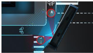
Sideguard Assist 2 is a safety assistance system that supports the driver in critical
