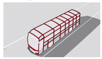
The strength of the bus/touring coach body is also an important factor for the level of passive safety of a bus/touring coach. Its resilience can mitigate the consequences of an accident. The high strength of our vehicles' bus/touring coach bodies is guaranteed in part by all-round, weight-optimised annular frames.
