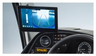
The 360° camera system consists of four cameras that capture the immediate vehicle environment and generate an indirect all-round view. The associated 10" screen is located on the A-pillar above the cockpit. This system allows pedestrians, cyclists and obstacles to be seen even in areas that are otherwise not visible to the driver. In this way, the system increases road safety, as collision hazards can be detected and, at best, prevented.
