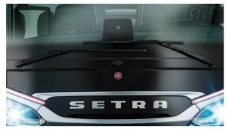
With its innovative profile, the flat wiper blade ensures that screen wash is evenly distributed on the windscreen. This increases comfort, saves screen wash and, due to the considerably better cleaning action, also ensures optimum visibility – ultimately a plus for safety.
