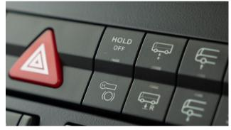
The electronic brake with hold function combines easier handling, more comfort and greater safety. When the bus is at a standstill, the vehicle is held by the service brake by pressing the brake pedal above a certain point, and the brake is automatically released when starting off. The function can be deactivated by a button.
