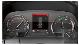
The wireless tyre pressure monitoring with indication in the multifunctional display is an electronic safety system that permanently monitors the air pressure of all tyres. Tyre pressure losses are displayed within the system limits.
