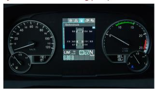
The right tyre pressure contributes to driving safety and significantly reduced fuel consumption. Even a tyre pressure set 0.5 bar too low can increase fuel consumption by up to 5%. The wheel electronics are positioned on the valve on the inside of the rim. The sensors record the data relevant to the tyre pressure and transmit it to the display instrument.
