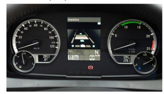
With the aid of a camera system behind the windshield, the Lane Departure Warning system detects when the vehicle unintentionally leaves a marked lane. As soon as the vehicle crosses the markings, the driver is warned by a clear vibration on the corresponding side of the driver's seat.
