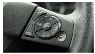
The Adaptive Cruise Control (ACC) with Active Brake Assist 6 (ABA 6) relieves the driver of the unnecessary stresses associated with maintaining a constant distance from the vehicle ahead, with a continuous measurement. ABA 6 additionally supports the driver in case of an imminent collision with stationary objects, moving objects and moving pedestrians.
